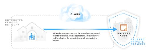
With VPNs, remote users are connected from their untrusted network to the trusted network to gain access to private apps
