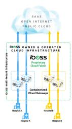
According to the <u>Google Transparency Report on HTTPS</u> 99% of all browsing time is over encrypted HTTPS connections. This requires connections to be decrypted by the SASE service to inspect content for malware, infections and data loss. To decrypt, special private key files must be used that allow traffic to be inspected and those key files must be available to the cloud gateways performing the inspection.
