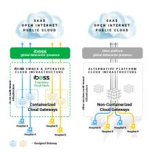
With alternative SASE platforms that lack containerization, network traffic from multiple organizations are processed within the same gateways that proxy, decrypt and firewall data for other organizations. Mixing data within the gateways that perform functions like decryption not only results in latency but increases security risks.
